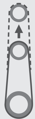
Dimensione nastri abrasivi (sviluppo) 2620-3250mm Abrasive belt (length) 2620-3250mm Hiomanauha (pituus) 2620-3250 mm
