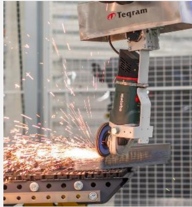
Heat-affected zone removal (HAZ)
