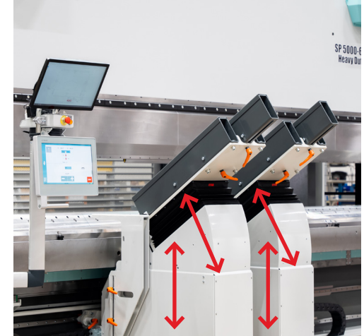
Movement by electrical cylinders, manual adjusting between programs not needed
