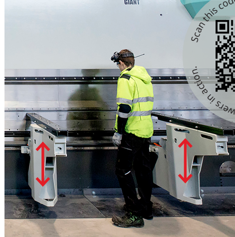
Vertical adjustment lightened with gas cylinder
