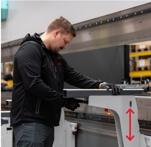
Vertical adjustment lightened with gas cylinder
